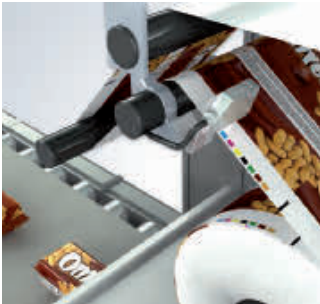
Reliable detection of standard or semi-transparent marks at normal or high speed
